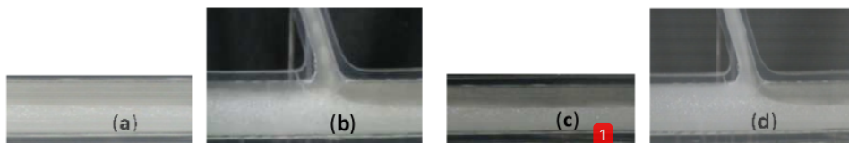
Figure 5. Flow pattern at the inlet STMI (a), at the T-junction 3L-13 (b) for J_w = 0.20 m/s, J_k = 0.14 m/s and flow resistance R_2 (5743 Pa), Flow pattern at the inlet STMI (c), at the T-junction 3L-3 (d) for J_w = 0.20 m/s, J_k = 0.14 m/s and flow resistance R_3 (6471 Pa), all for \theta = 60^\circ
