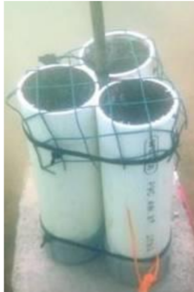
Figure 2. Modified sediment trap design (Windusari et al., 2015)
