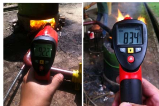
Figure-4. Measurement by means of infrared Thermogun.
