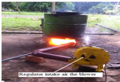
Figure-3. The complete installation of a simple furnace system.
