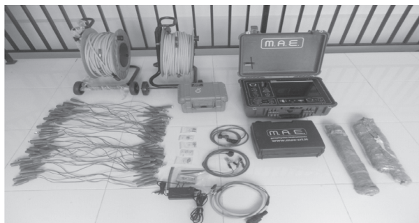
Fig. 3. MAE Geoelectric tool unit used with 144 meters cable length
