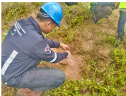
Figure 7. Sampling of embankment soil
