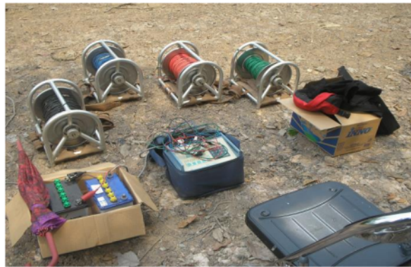
Figure 2. Geoelectric Tool Model-2115 McOhm and its accessories (Ibrahim, 2006)
