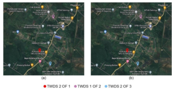
Figure 2. Comparison of Calculation Results of the p-Median Problem a) Using LINGO 13.0 and b) Myopic Algorithm with Maximum Distance of 500m
