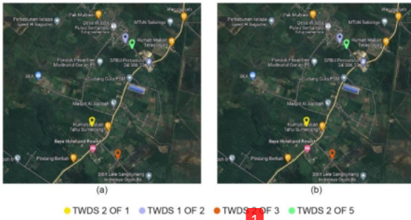
Figure 1. Comparison of Calculation Results of the p-Median Problem a) Using LINGO 13.0 and b) Myopic Algorithm with Maximum Distance of 500m
