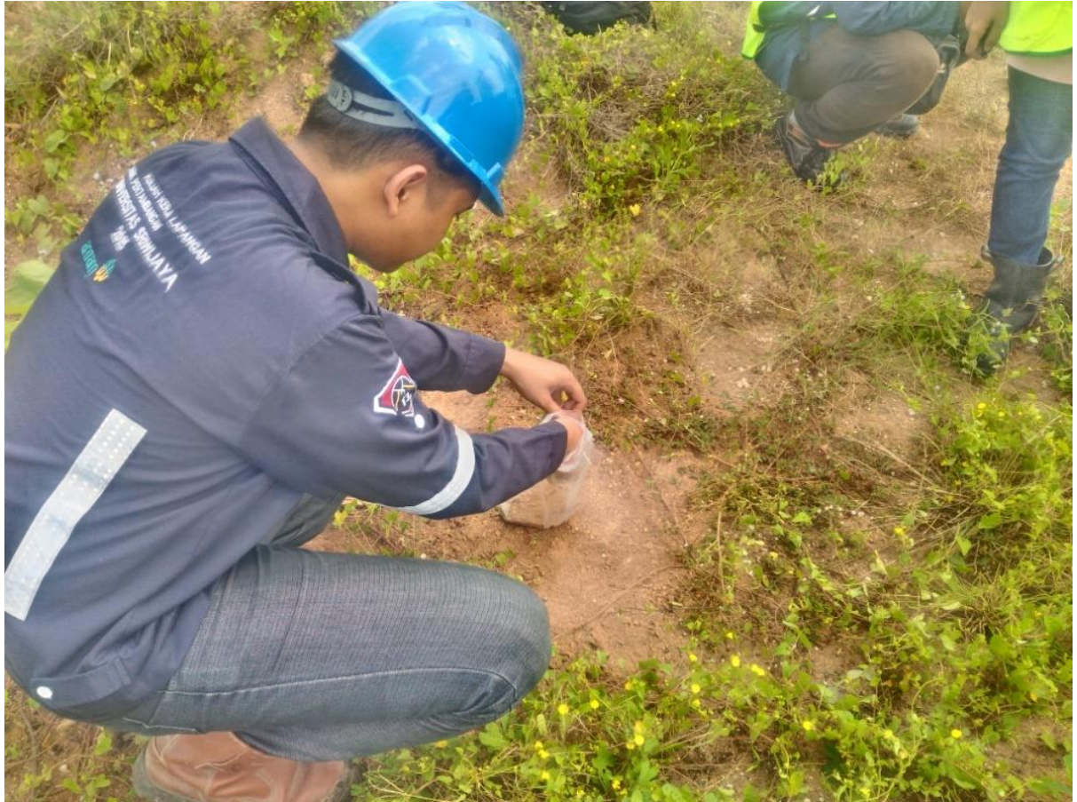
Figure 7. Sampling of embankment soil
