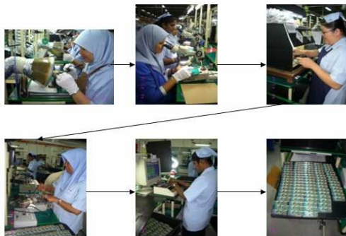
Fig.2. The works sequence to assemble complete TV tuner Data Gathering and Analysis
