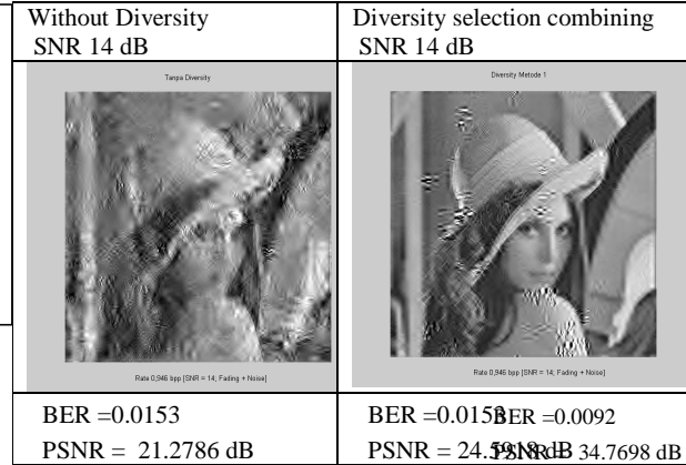
Figure 4. Comparison result of image reconstruction between using diversity and without diversity for SNR 14 dB
