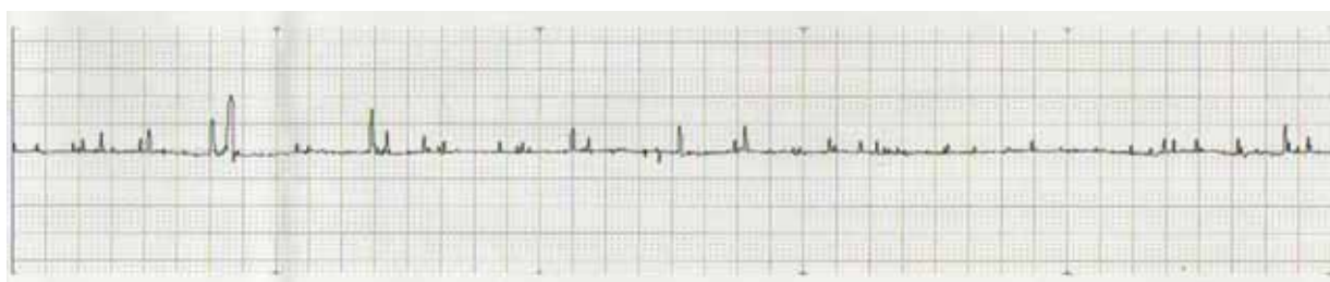
Figure 5. Surface profiles of CAE PVD coatings at -100 V ( EVA-L = 4.0 \text{ mm} , \lambda c = 0.8 \text{ mm} \times 5 ).
