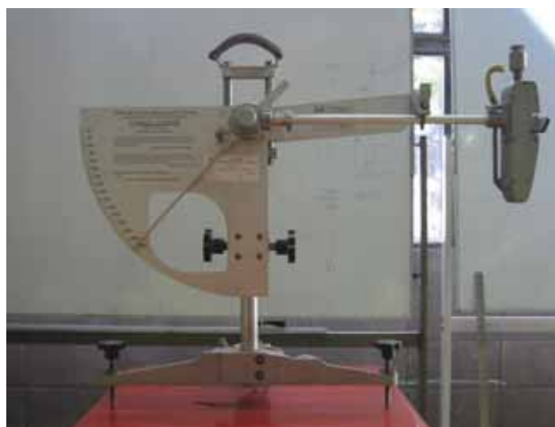
Figure 3: Skid resistance test
