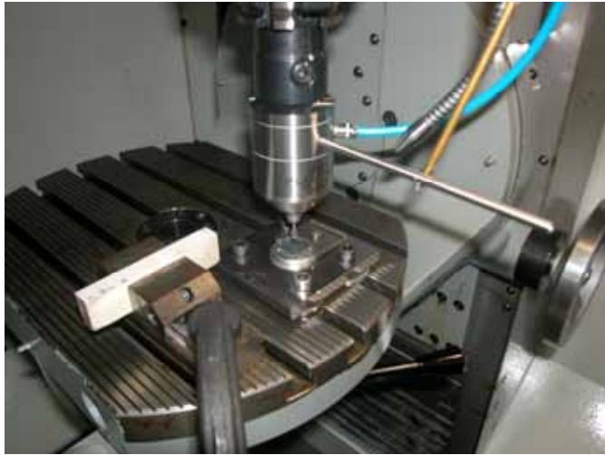
Figure 1: The experimental set-up showing a high-speed jig grinder unit attached on NC vertical milling spindle and the Al 2 O 3 abrasive stick (grade Nr.2).
