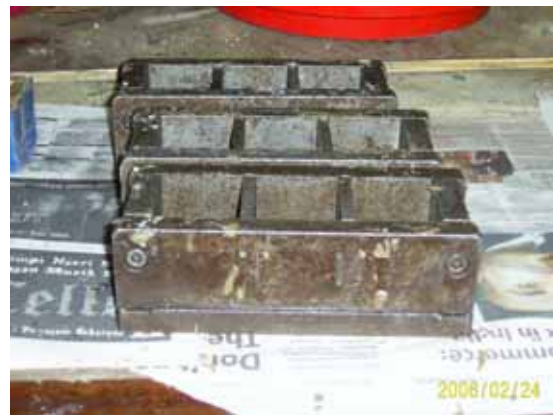
Fig. 2: Steel mould for casting cube
