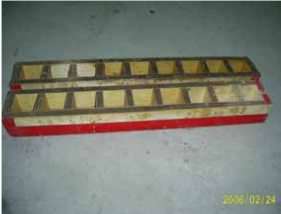
Fig. 3: Timber mould for casting cube
