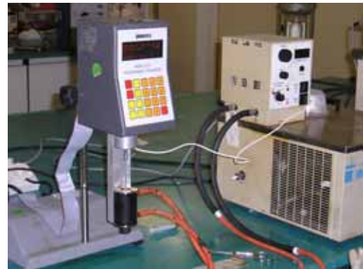
Fig. 4: Measure of resin grout's viscosity by Brookfield rotational viscometer
