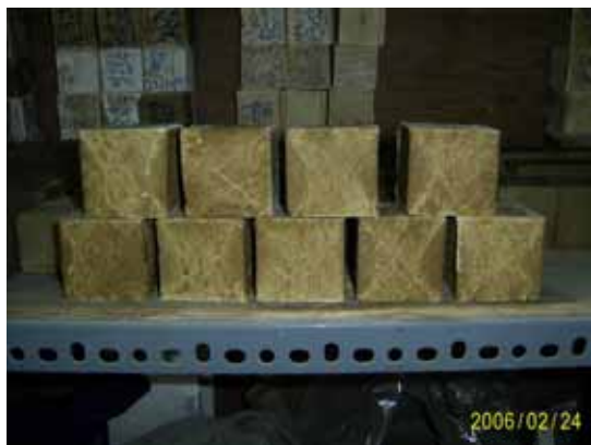
Fig. 7: Failure mode of epoxy grout cubes after compressive test
