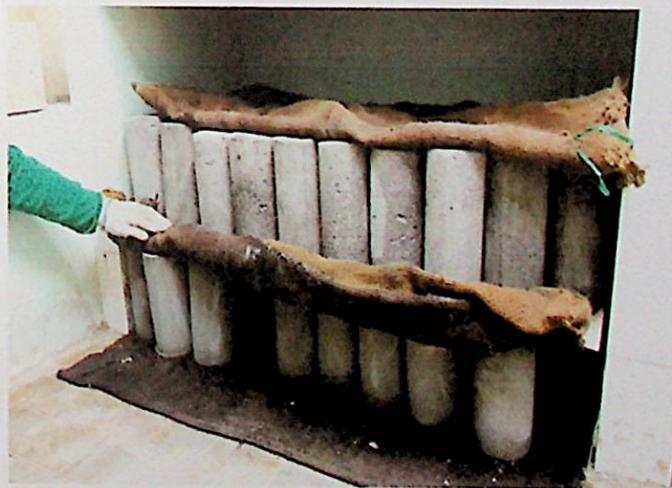
Gambar 3.23. Proses *curing* beton
