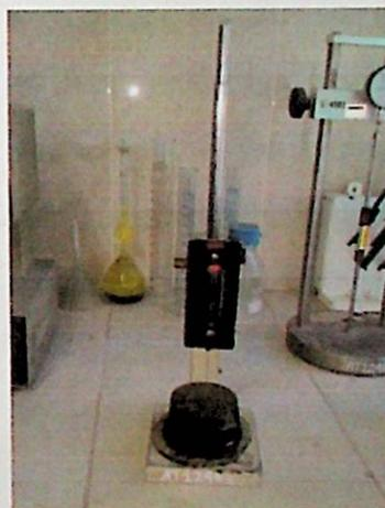
Gambar 3.21. Proses pengujian *setting time*
