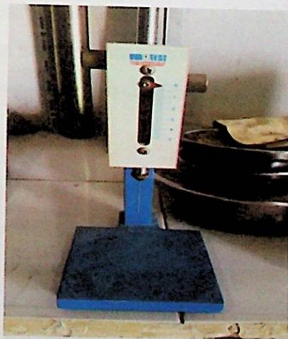
Gambar 2.7. Alat uji *setting time*
