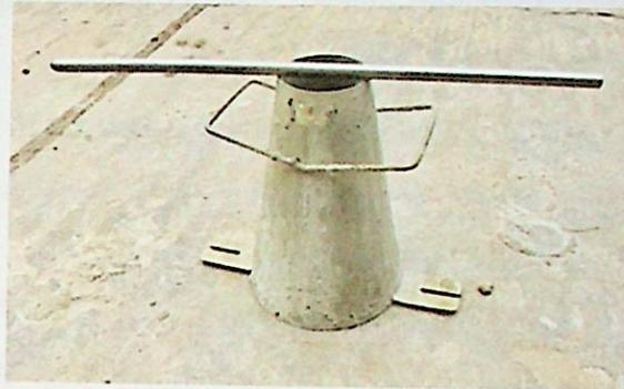
Gambar 2.6. Alat uji *slump flow*
