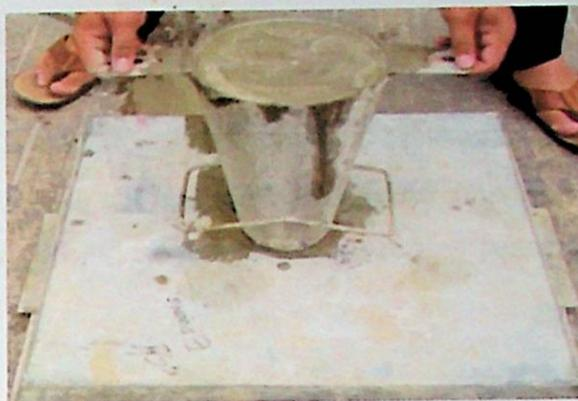
Gambar 3.20. Proses pengujian *slump flow*
