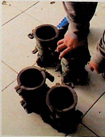
Gambar 3.9. Bekisting benda uji
