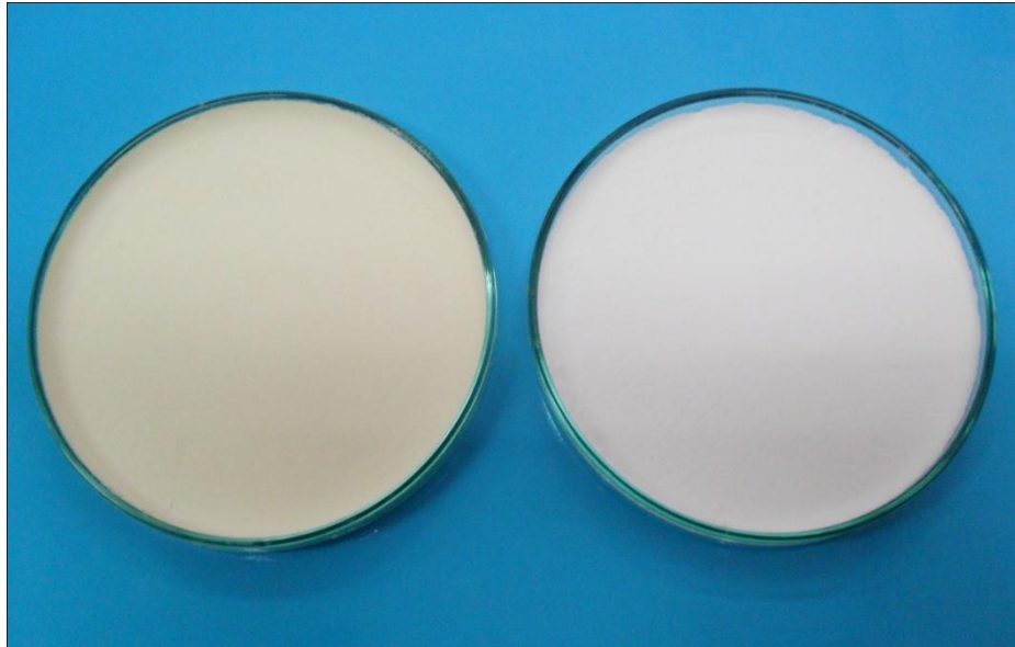
(A) banana peel cellulose (B) Commercial cellulose Figure 1 : Color of BPC (A) compared to commercial cellulose (B)
