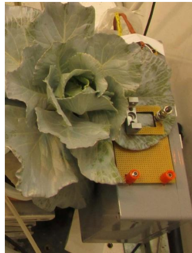
Figure 2: A view of the experimental plant and the leaf clamping system on the laser speckle imaging apparatus placed inside the chamber.
