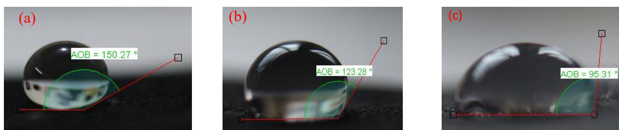
Figure 5. Digitalized photograph of water bubble for measuring the contact angle between water and the surface of (a) conductive paper (b) gas diffusion layer with carbon vulcan and (c) gas diffusion layer with carbon dot on conductive paper.
