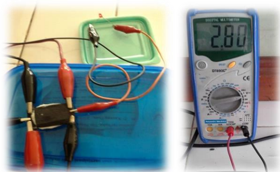
Figure 2. (a) Supercapacitor that has been made and installed with LED lights (b) Measurement tool for a circuit using a supercapacitor.
