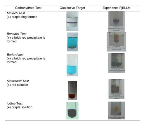
Figure 2. Qualitative test of carbohydrates in apple juice
