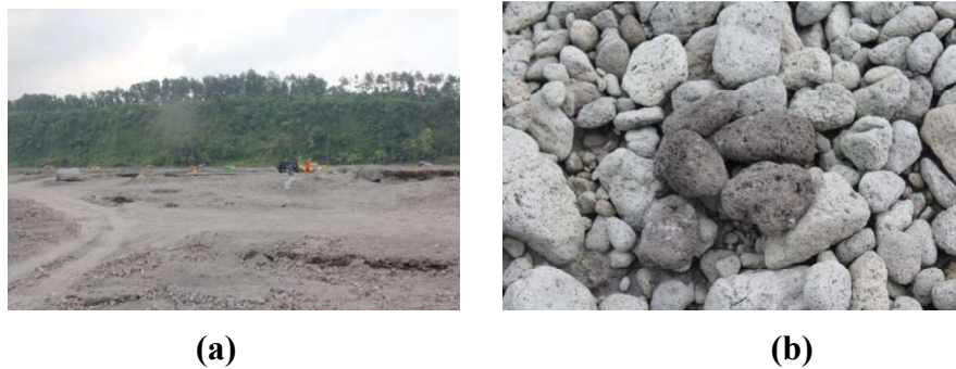
Figure 1 Deposit of scoria and pumice:(a)Kali Putih River near Mount Kelud (b)Visualization of scoria (dark color) and pumice (light color)
