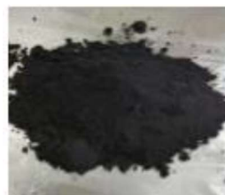
Figure 2. Final result, the active carbon made from Agave fiber
