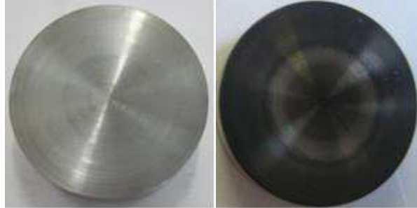
Figure 1 Comparison of AISI-316L specimen before and after plasma nitriding. (a): sample before nitriding, and, (b) after nitriding at 480 °C for 7.2 ks.
