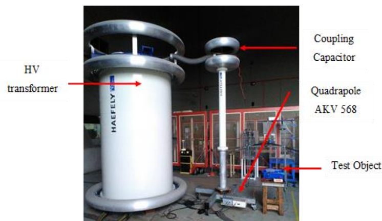
Figure 3. Haefely's partial discharge measurement setup
