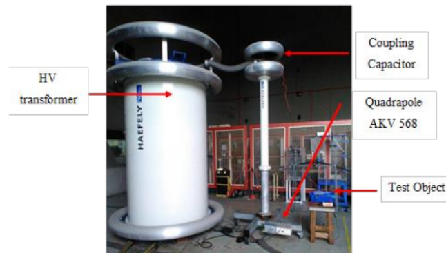
Figure 3. Haefely's partial discharge measurement setup
