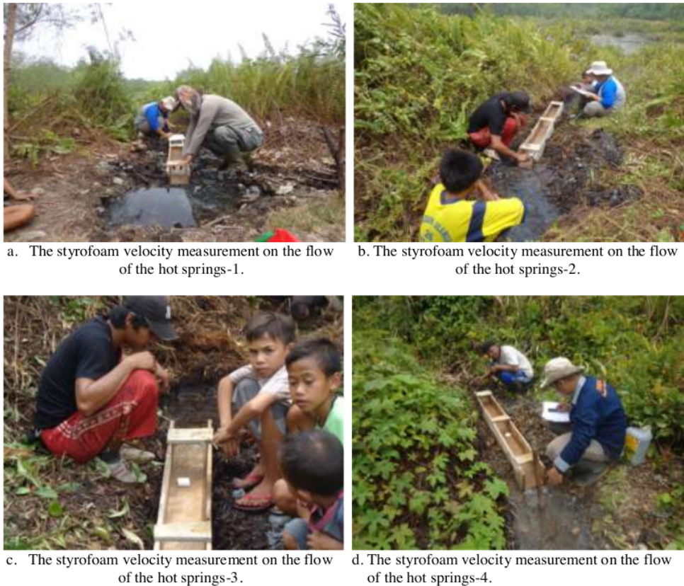
Fig. 3.1: The styrofoam velocity measurement on the flow of the hot springs.
