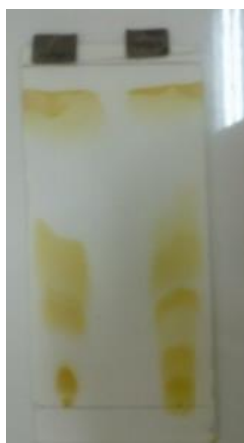
Figure 2. Chromatogram of TLC Ethanolysis Product (Ethanolysis Product from Ketapang Seed Oil ) (I) and (II) Ketapang Seed Oil
