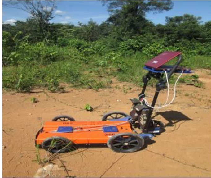
Figure 2. Georadar OKKO with frequency of 250 MHz
