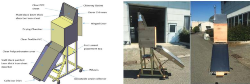
Figure 3. Type of indirect solar dryer
