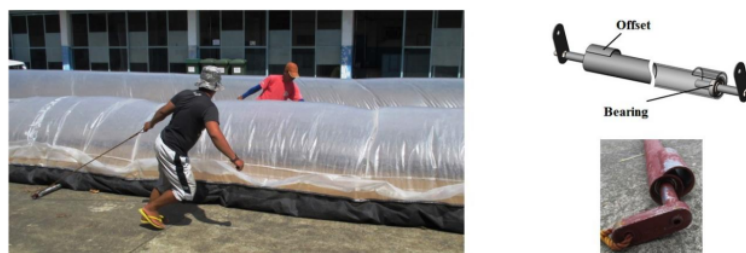
Figure 10. Roller for the admixture of the grains
