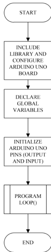
Figure 2. Flow chart of the Main Program
