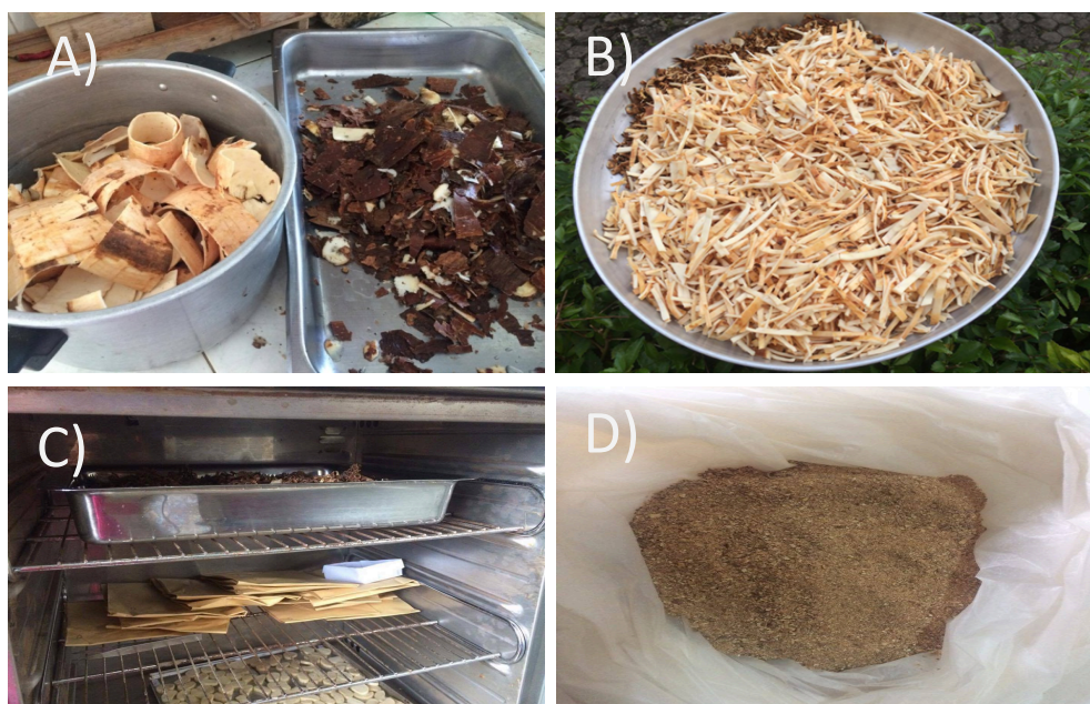
Figure 1. Preparation of cassava peel sample consisted of washing, cutting, drying and grinding process.
