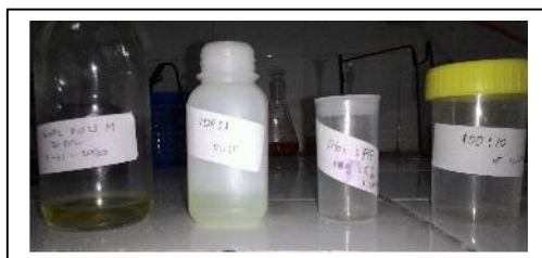
Figure 1. Results of Sol-Gel-Varying concentrations from left to right with a concentration 100%, 100%: 1%, 100%: 5%, and 100%: 10%
