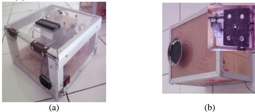
Figure 3. Low-frequency vibration generators.
