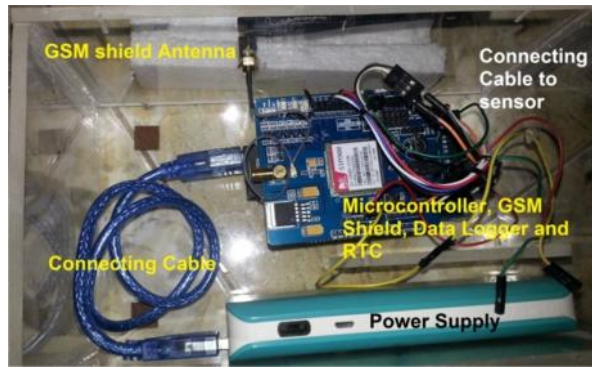
Figure 3. A prototype of data acquisition system.
