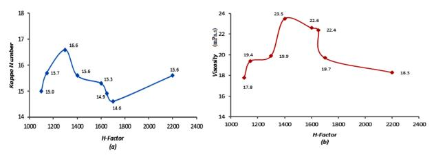
**Figure 3.** (a) Relationship between H-Factor and Kappa Number, (b) Relationship between H-Factor and Viscosity at a Production rate of 1300 ADT/d
