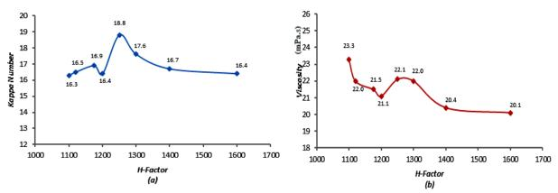
Figure 4. (a) Relationship of H-Factor and Kappa Number, (b) Relationship of H-Factor and Viscosity at a Production rate of 1400 ADT/d
