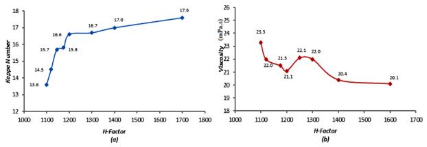
**Figure 5.** (a) Relationship of H-Factor and Kappa Number, (b) Relationship of H-Factor and Viscosity at a Production rate of 1500 ADT/d
