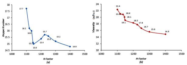
Figure 6. (a) Relationship of H-Factor and Kappa Number, (b) Relationship of H-Factor and Viscosity at a Production rate of 1600 ADT/d
