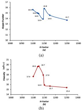
Figure 2. (a) Relationship between H-Factor and Kappa Number, (b) Relationship between H-Factor and Viscosity at a Production rate of 1200 ADT/d
