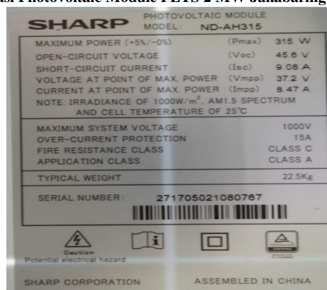
Gambar 3. 2. Data Name Plate Photovoltaic Module PLTS 2 MW Jakabaring
