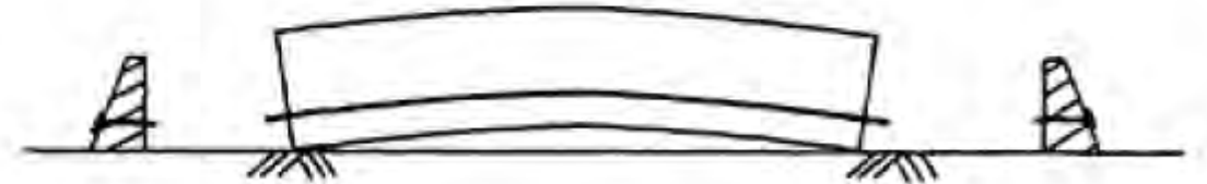
(c) Tendons released and prestress transferred
