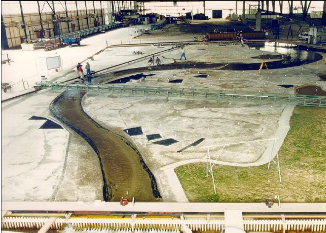
Model fisik sungai Grensmaas (WL | Delft Hydraulics), 1:60
