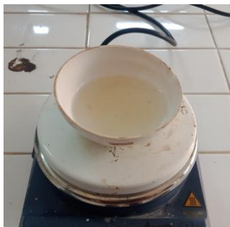
Gambar 25. Proses Penguapan TDS ( Total Dissolved Solid )
