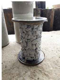
Gambar 3.25. Capping Pervious Concrete
