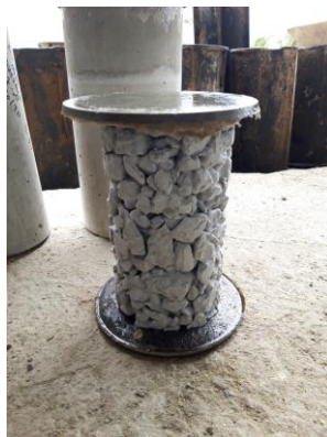
Gambar 3.25. Capping Pervious Concrete
