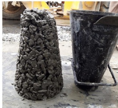
Gambar 4.1. Hasil pengujian slump pervious concrete
