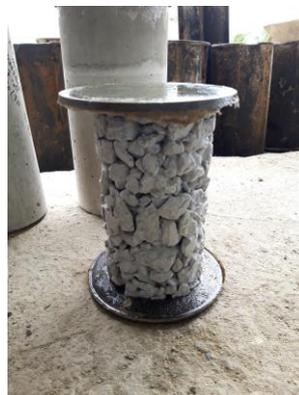
Gambar 3.25. *Capping Pervious Concrete*
