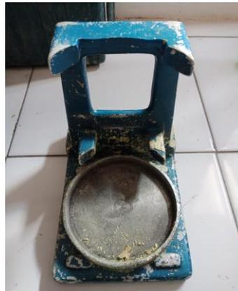
Gambar 3.17. *Vertical cylinder capping set*
