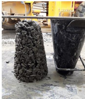
Gambar 3.22. Uji *Slump Pervious Concrete*
