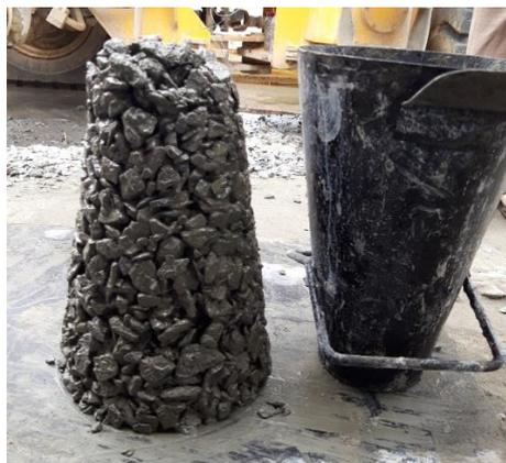
Gambar 4.1. Hasil pengujian *slump pervious concrete*
