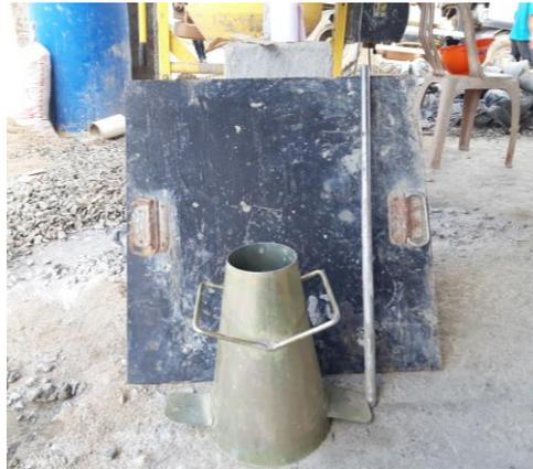
Gambar 3.15. *Slump Cone*
