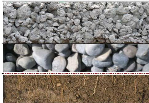
Gambar 2.2. Lapisan Pada *Pervious Concrete* (Sonebi et al, 2016)
