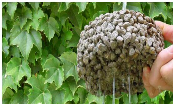
Gambar 2.1. *Pervious concrete* (Jj Harison, 2016)
