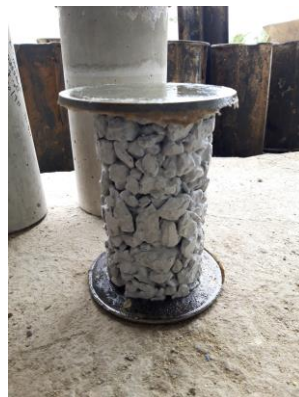
Gambar 3.25. Capping Pervious Concrete
