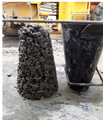
Gambar 3.22. Uji Slump Pervious Concrete
