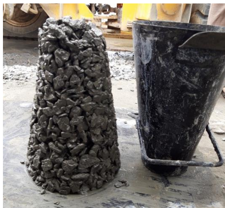
Gambar 4.1. Hasil pengujian slump pervious concrete
