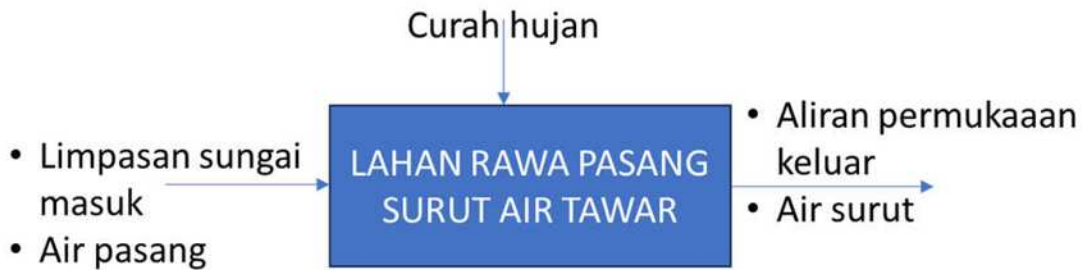
Gambar 13. Diagram input-output air lahan rawa lebak pasang surut
