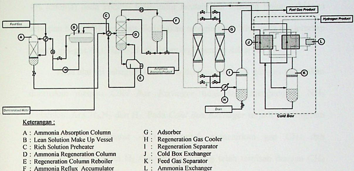
Gambar 3.2. Blok diagram Unit PGRU (*Purge Gas Recovery Unit*).
