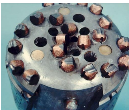
Gambar 2.19 Diamond Core Drilling
