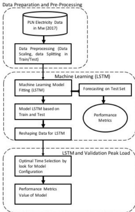
Fig. 2 Proposed forecasting methodology in LSTM
