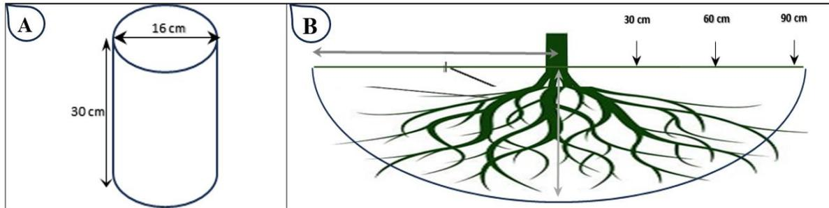
**Figure 2.** Sample ring size (A) and root sampling points (B).
