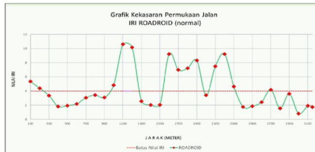
Figure 2. Surface Roughness Graph of Alamsyah RPN street for normal direction ( Roadroid )
