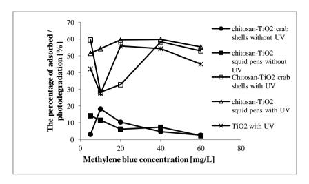
**Figure 4.** The concentration vs percentage of photodegradation of methylene blue by nanocomposite chitosan-TiO<sub>2</sub> and TiO<sub>2</sub> with and without UV irradiation.
