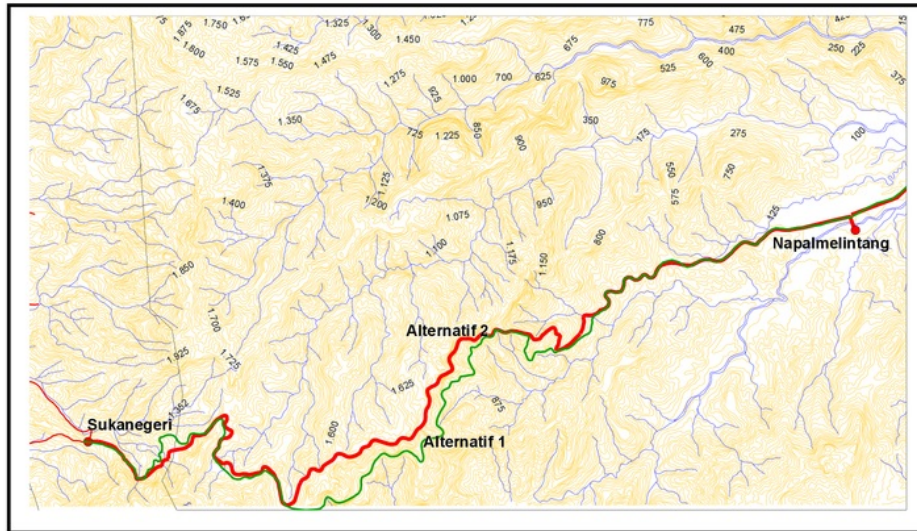
Figures 2. The two road layouts (Alternative 1 represented in green and 2 in red)
