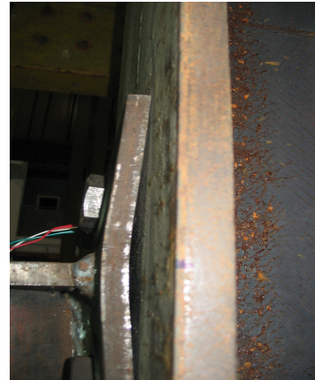
Figure 8 Deformation of end-plate for N7 specimen (E3R20)
