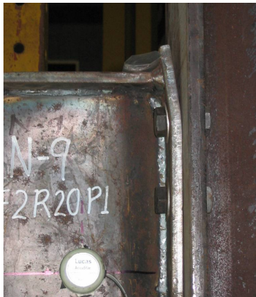
Figure 7 Deformation of end-plate for N9 specimen (F2R20)
