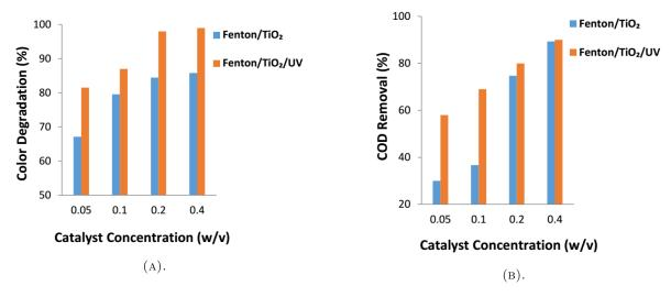
FIGURE 2. Effect of TiO<sub>2</sub> catalyst concentration on (a) RR 2 colour degradation and (b) COD removal by Fenton/TiO<sub>2</sub> and Fenton/TiO<sub>2</sub>/UV methods (Fenton reagent molar ratio of 1 : 80, RR 2 concentration of 150 ppm, pH 3, reaction time of 5 min).
