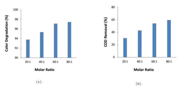
FIGURE 1. Effect of Fenton reagent molar ratio on (a) RR 2 colour degradation (b) COD removal by using Fenton/UV method (RR 2 concentration of 300 ppm, pH 3, reaction time 5 min).
