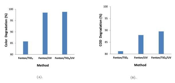
FIGURE 3. (a) RR 2 colour degradation and (b) COD removal by Fenton/TiO<sub>2</sub>, Fenton/UV, and Fenton/TiO<sub>2</sub>/UV methods (Fenton reagent molar ratio of 1 : 80, RR 2 concentration of 150 ppm, TiO<sub>2</sub> concentration of 0.4%, pH 3, reaction time of 5 min).
