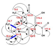
**Fig 5.** The HMBC and COSY correlations of 7hydroxy-3,4,5-trimethyl-6-on-2,3,4,6-tetrahydroisoquino line-8-carboxylic acid (1) (arrow bent for HMBC correlations and bold line for COSY correlations)
