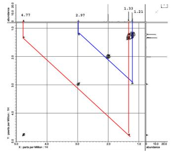
**Fig 4.** The COSY spectrum of compound 1 showed correlation between methine proton H-4 ( $\delta_H$  2.97) with methyl proton 4-CH<sub>3</sub> ( $\delta$ H 1.21) and methine proton at  $\delta_H$  4.77 with methyl proton 4-CH<sub>3</sub> ( $\delta_H$  1.33) (<sup>1</sup>H-500 MHz; <sup>13</sup>C-125 MHz, CDCl<sub>3</sub>)
