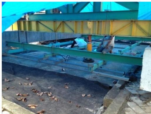
Figure 3 Loading test on the edge of slab
