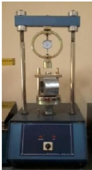
**Picture 1.** Analog Marshall Test
