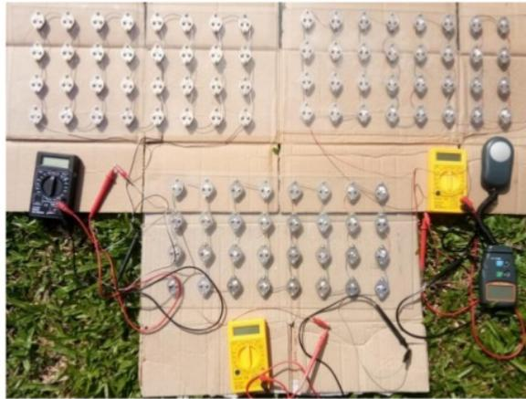
**Gambar 4.2** Pengujian Prototipe Panel Surya Berbasis Transistor 2N3055
