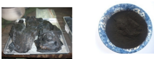
Figure 1. Coal result before and after physical and chemical activation
